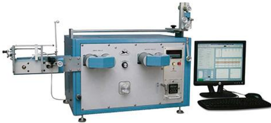
Figure 6: LH-402 Dynamic Tensile Tester
