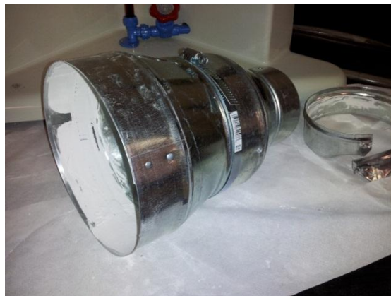
Figure 58 Partial dryness of the resin
