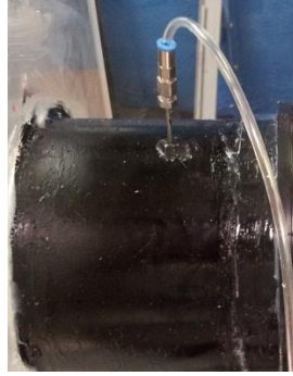
Figure 70 Pitot tube placement
