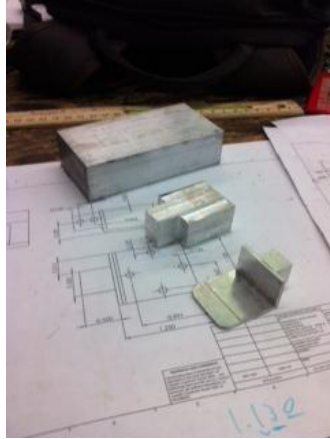
Figure 55: Motor Support Transformation
