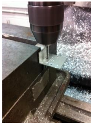
Figure 56: Motor Support Drilling
